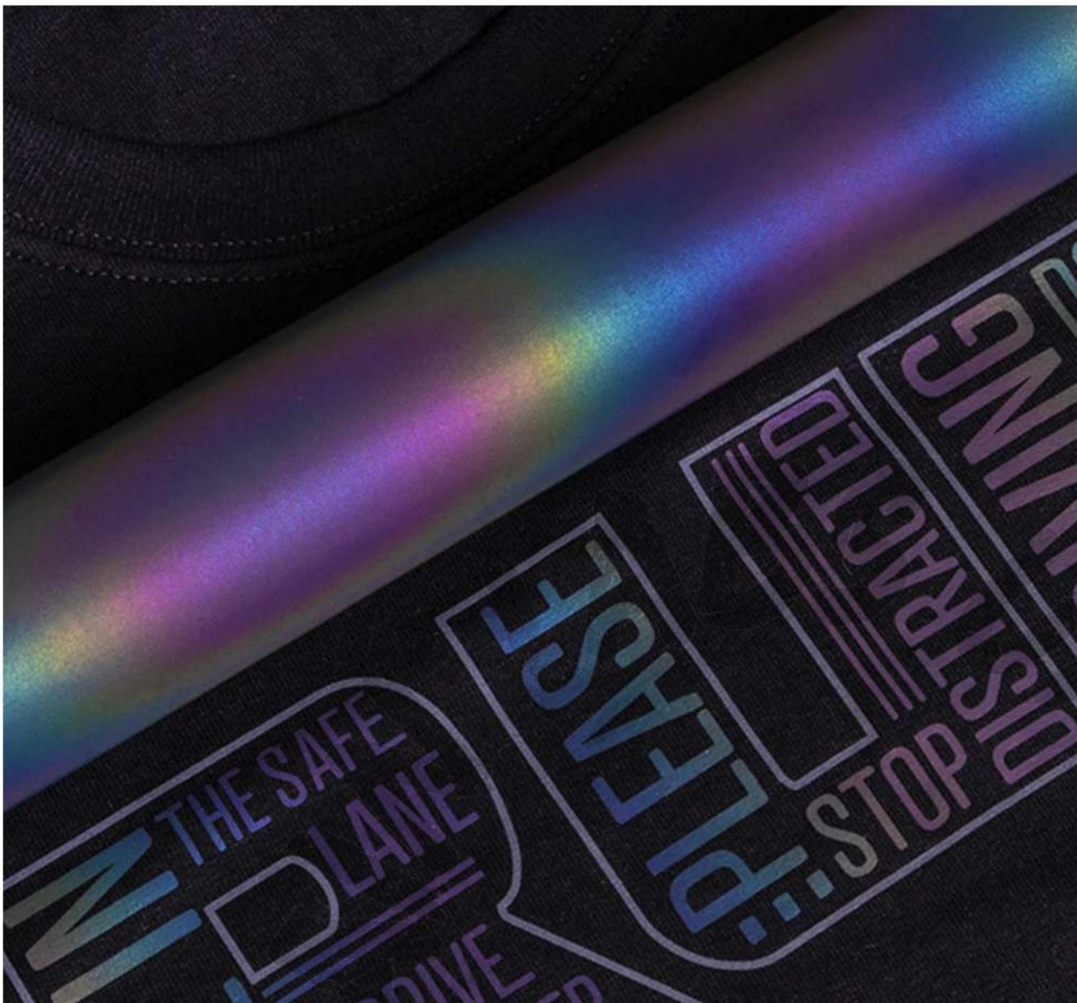
**EasyReflective** is a highly reflective HTV specifically designed for applications that require high visibility having a one-step application at 150°C/15 sec and 3,5 bar. The sticky adhesive carrier helps cutting and weeding small graphics details. It is suited for 100% cotton, 100% polyester and poly/cotton blends, Elastan / Spandex.
